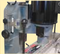
Adjustable height stop and depth stop
